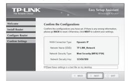
You can save these settings in a text file on your desktop. If you forget the Network Security Key, you can check the Router Settings.txt.
